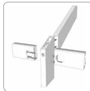
Eaves purlin - exploded view
